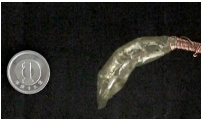
Fig. 1. Soft actuator for ultralow environment
