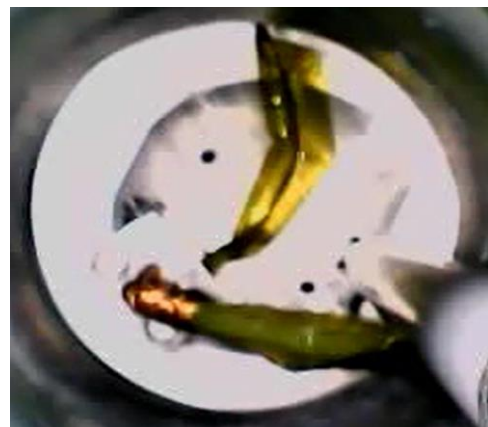
Fig. 2. Bending motion of soft actuator at liquid nitrogen temperature
